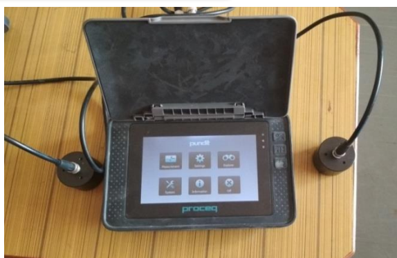
Figure 6.9 Ultrasonic Pulse Velocity Test
