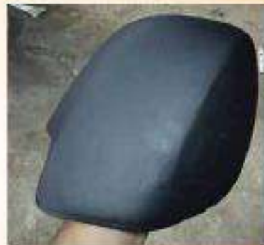
Prototype Automobile body panel developed using hybrid composite (Example: Car mirror shell)
