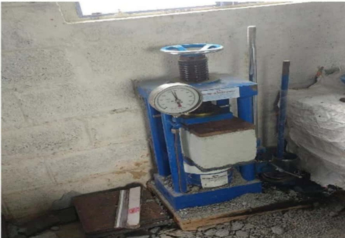
Fig 3.3 Compression test on concrete blocks
