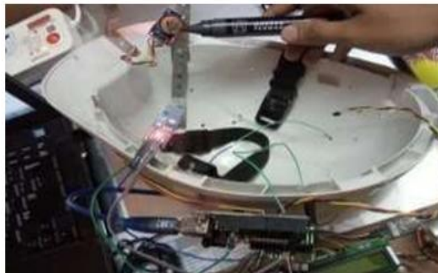
Fig 9.3 Alcohol Detection in Hemet Section
