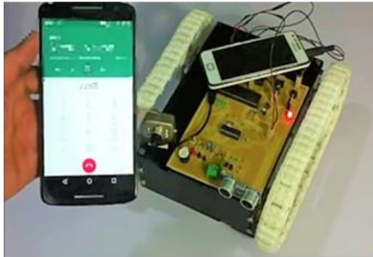
Fig 3: Cell Phone call controlled robot
