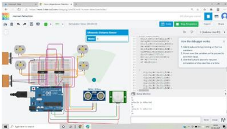
Fig. 5: Obstacle detected by Ultrasonic sensor rerepresented by using Tinkercad software
