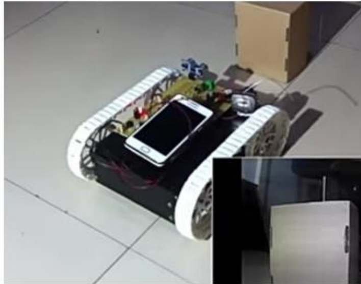
Fig 5: Ultrasonic obstacle detection
