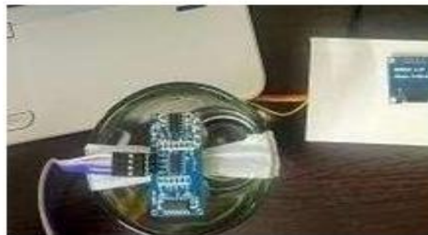
Fig.3: Ultrasonic sensor connection
