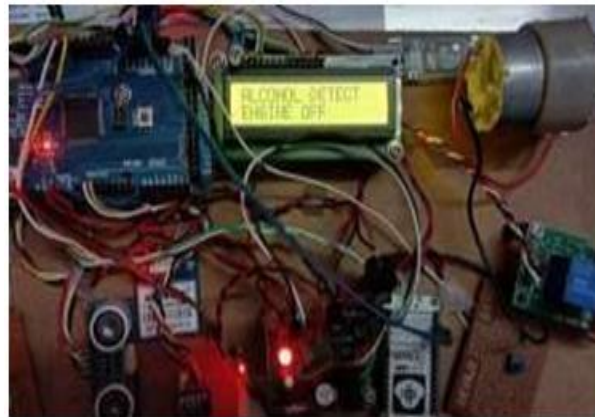
Fig 9.4 Alcohol Detected Engine off
