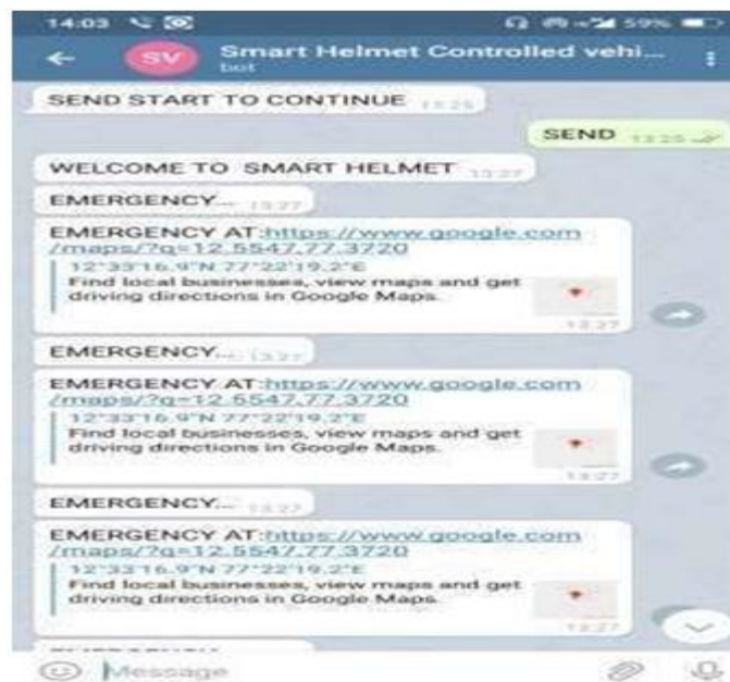
Fig. 9.8 Accident emergency message and live location
