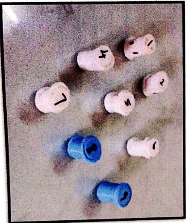
Fig. 4.6 Broken specimen of compression.
