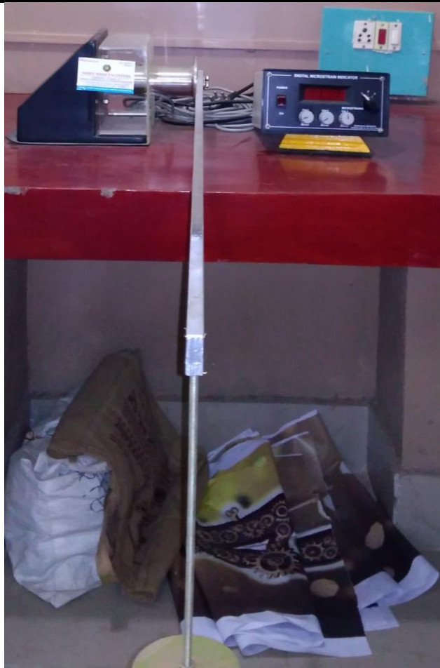
Fig: Strain gauge rosette experimental setup
