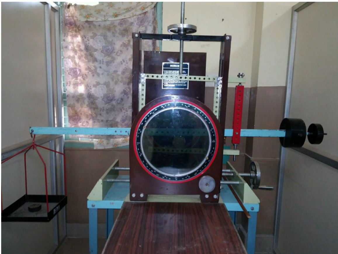
Fig: Circular polariscope experimental set up.
