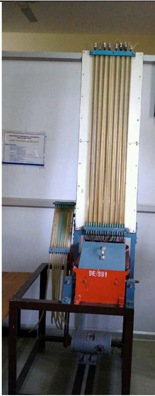
Fig: Slider bearing experimental set up.
