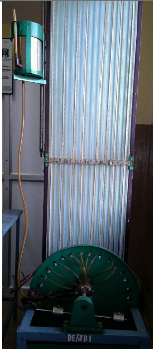
Fig: Journal Bearing experimental set up
