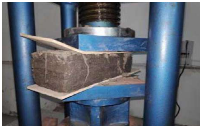
Fig: Compression strength test on brick to determine the load carrying capacity of bricks under compression
