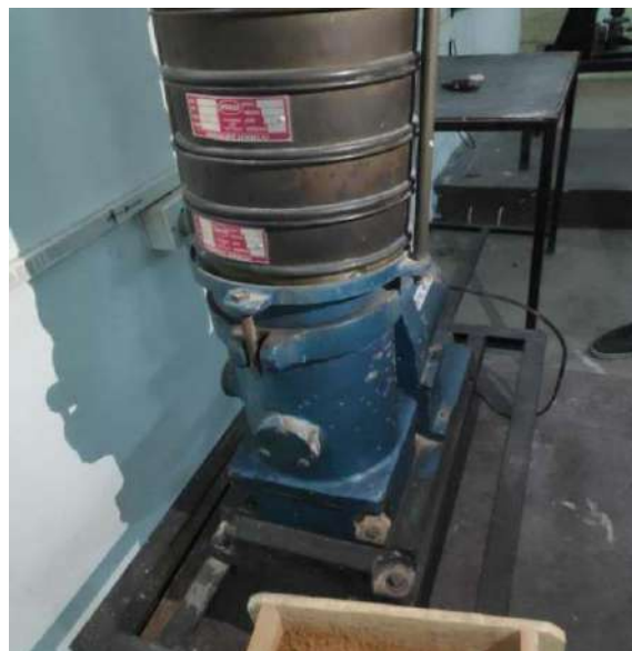
Fig: Sand sieving process on the sand sieving plastic(right) for the batching process
