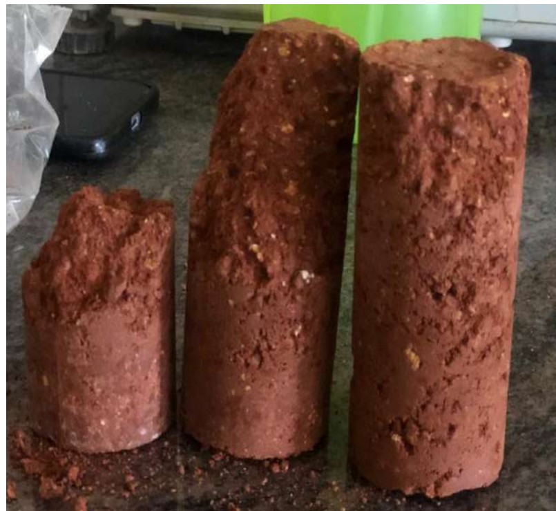
Fig.5.2.2 Unconfined compression test specimen after test.
