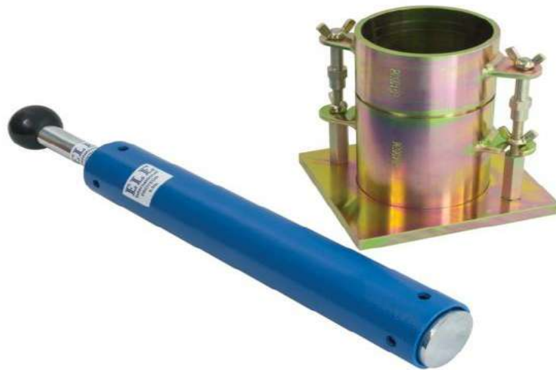
Fig.4.2 Compaction mould and rammer
