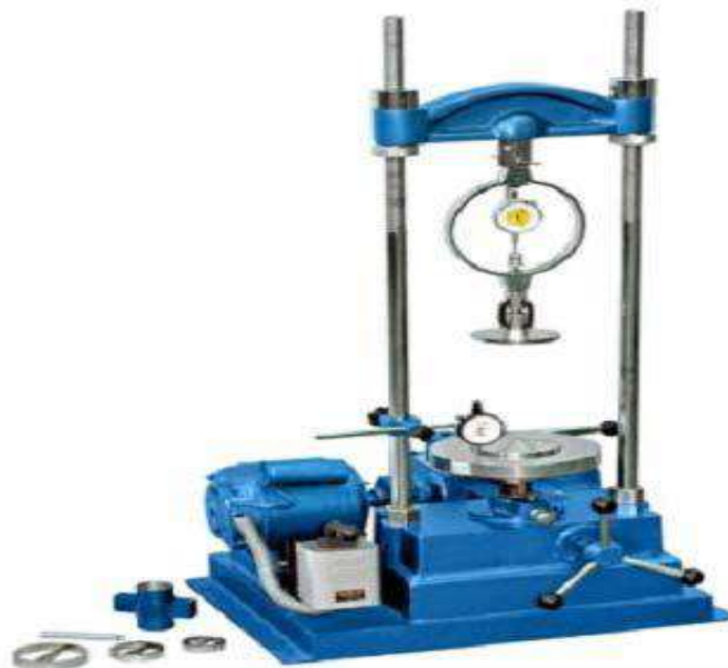
Fig.5.2.0 Unconfined Compression Strength Test
