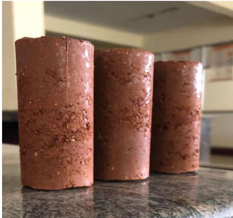
Fig.5.2.1 Unconfined compression test specimen before test.
