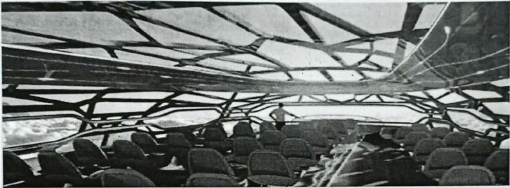
Cabin membrane:the lattice structure could be constructed using large-scale additive layer manufacturing techniques
