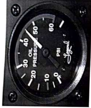
Fig 3.1 oil pressure indicator
