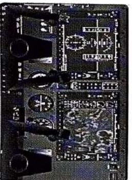
Figure 1b. This electrically operated flat screen display instrument panel, or glass cockpit, retains an analog airspeed indicator, a gyroscope-driven artificial horizon, and an analog altimeter as a backup should electric power be lost, or a display unit fails
