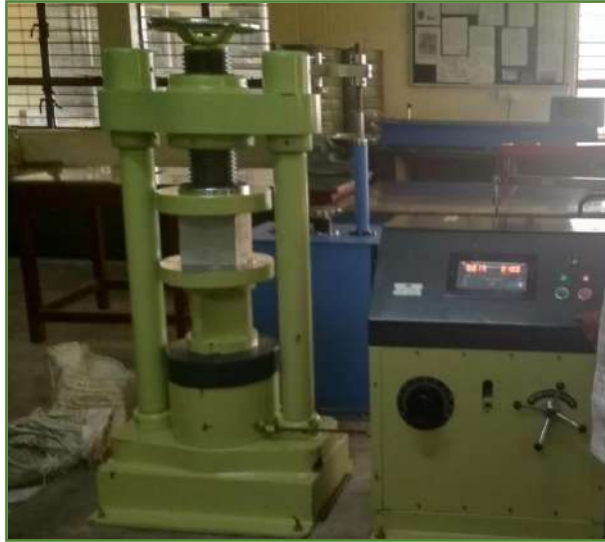
Figure 5.18 Digital Compression testing machine
