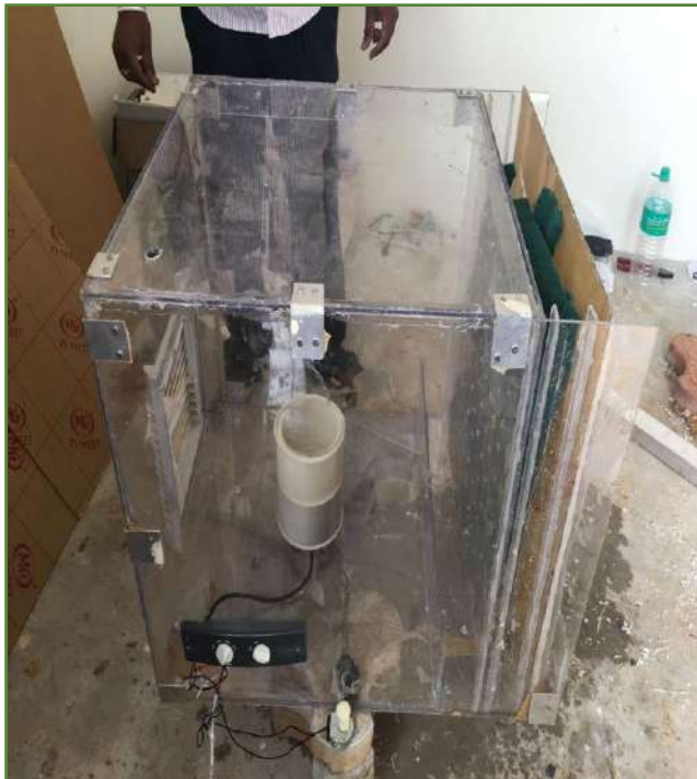
Figure 5.11 Model of air conditioning by geothermal heat pump
