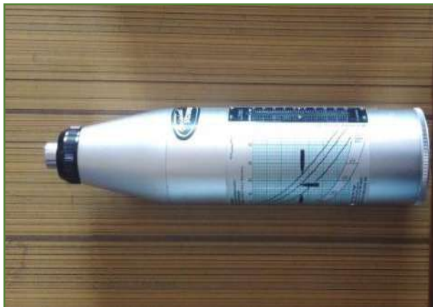
Figure 5.26 Rebound hammer (NDT)
