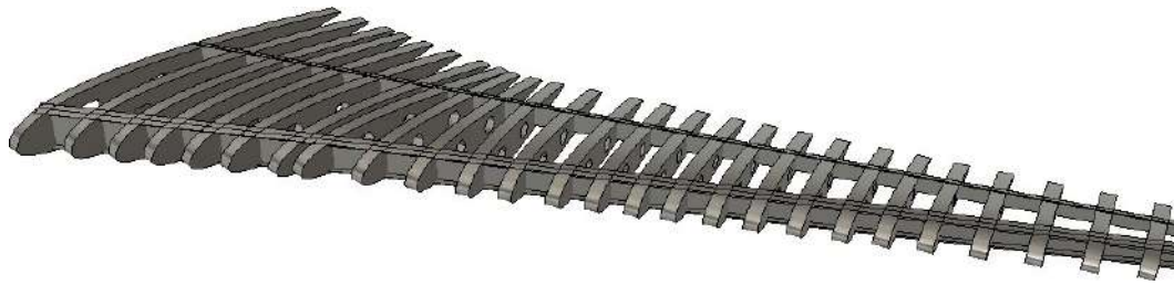
Fig 4.18. Giving thickness to ribs and spars.
