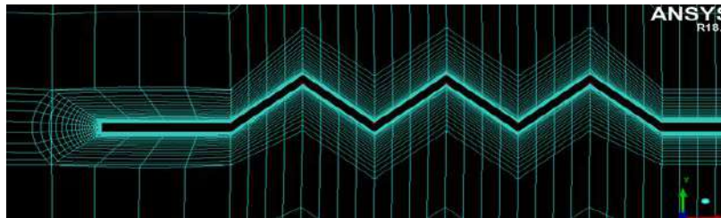
Fig 8.4: Mesh near the corrugations
